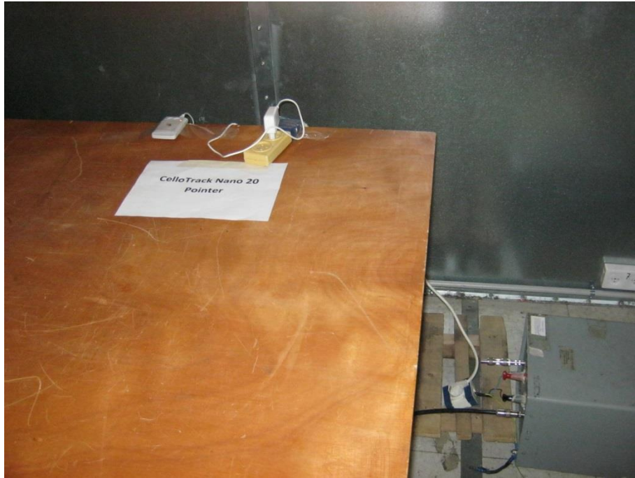
Figure 4. Conducted Emission from AC Mains Test
